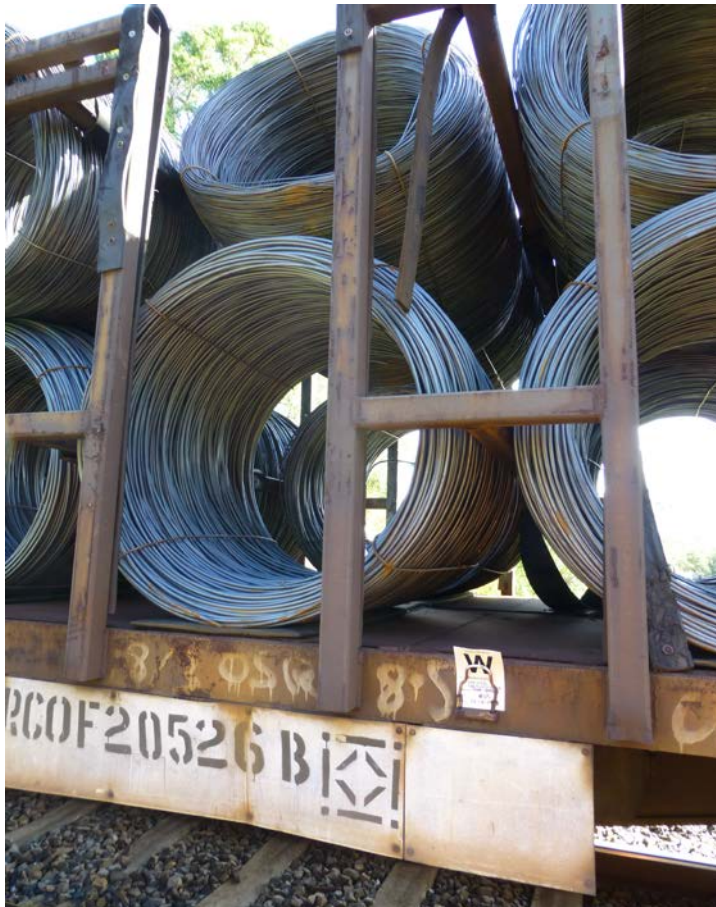
Figure 4: Loaded wagon RCOF20526B with shifted coils
